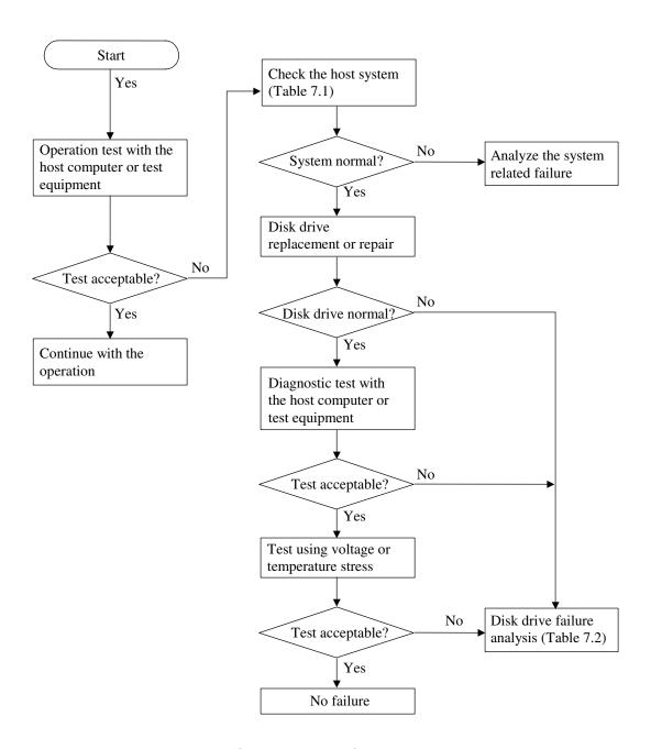
Figure 7.3 Test flowchart
